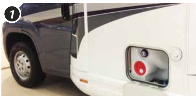
Fresh water tanks
